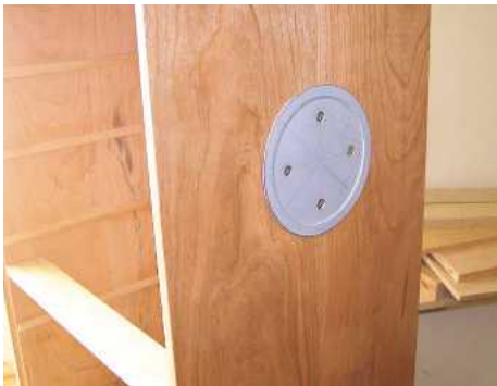
▲ Pic.23 ...and drilled the steel back plate so that it could be screwed to the side panels
